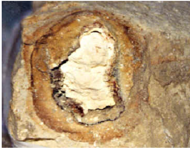
Close-up of an impact reveals an embedded sulfur ball.
